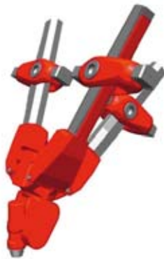
Parallel kinematic type Exechon
